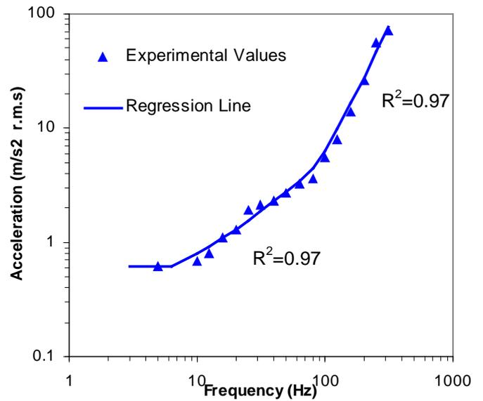
**Figure 6d.** Annoyance Threshold Test
