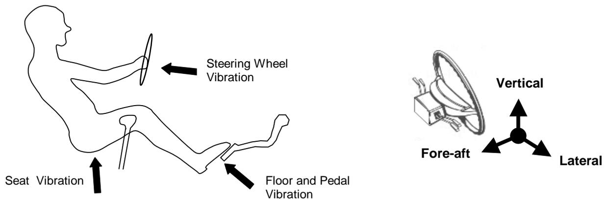
**Figure 1a)** Main sources of vibration disturbances in a vehicle. **1b)** Axis of vibration on a steering wheel
