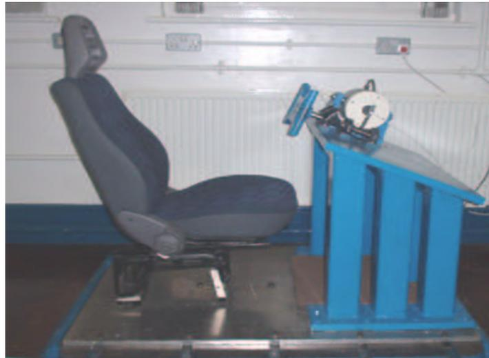
**Figure 2.** Steering wheel rotational vibration test rig.
