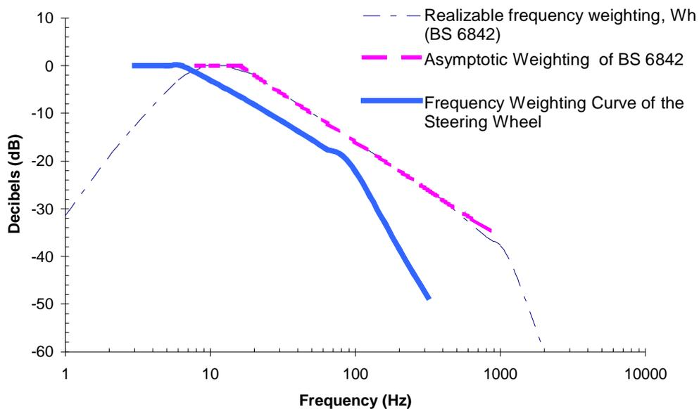
**Figure 7.** Asymptotic weighting curve of rotating steering wheel,  $W_s$  and asymptotic weighting of the hand,  $W_h$  taken from BS 6842
