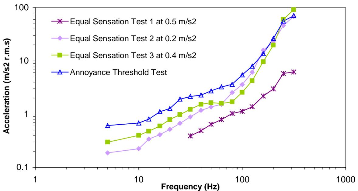
**Figure 5.** Mean experimental values of the equal sensation tests and annoyance threshold test for 30 subjects.
