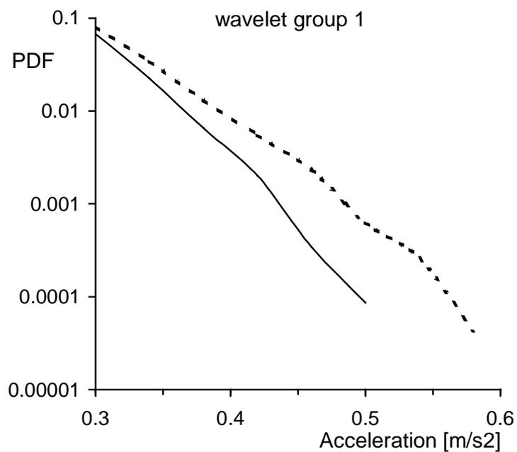
Figure 2) Seat guide vertical acceleration PDF tail for a road signal (- -) and for its mission signal constructed by means of the method of classical Fourier Series inversion (—)
