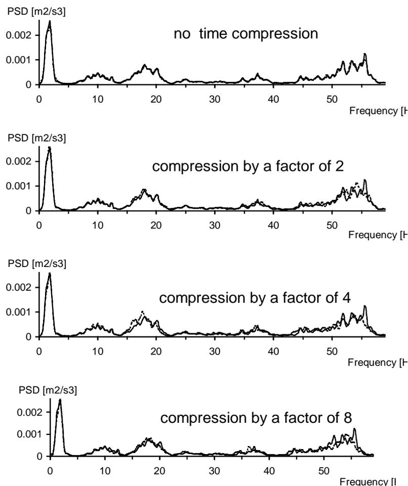
Figure 10) PSD comparison between the final mission signals (- - -) for the seat guide vertical acceleration data and the original road data (—) for compression ratios of 1, 2, 4 and 8.
