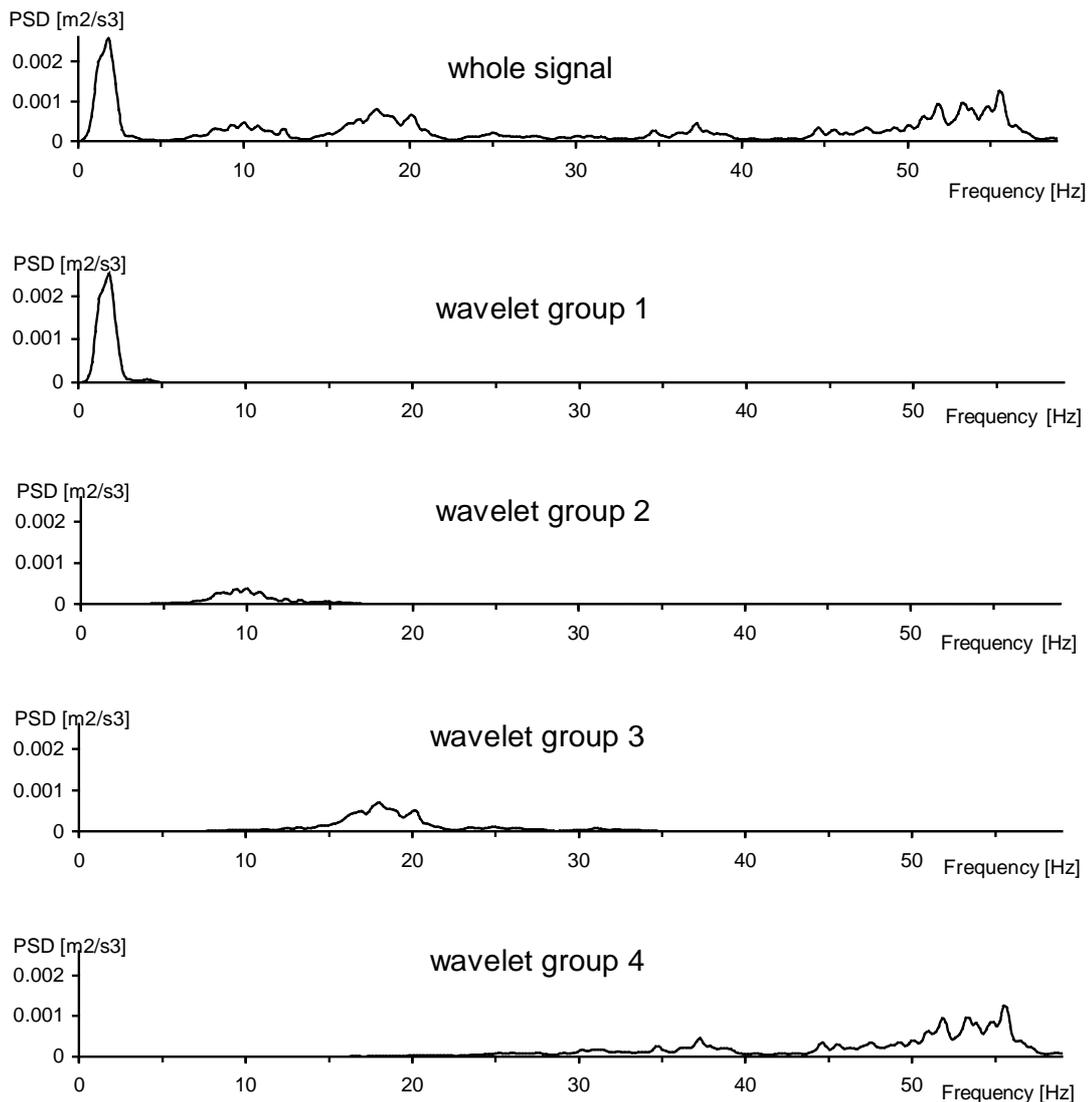
Figure 4) Example of the wavelet grouping procedure applied to seat guide vertical acceleration data. The wavelet levels in the frequency range from 0 to 60 Hz were organised into 4 groups.
