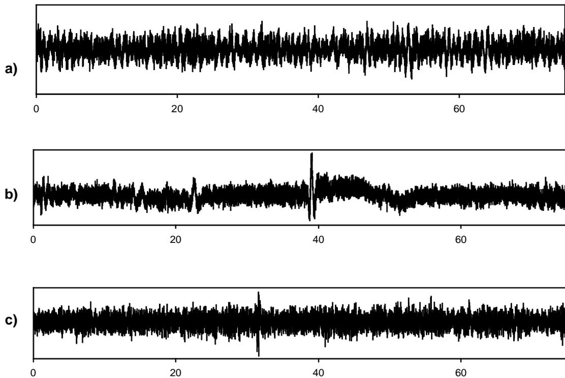
Figure 1) Seat guide vertical acceleration data produced by three road surfaces.
