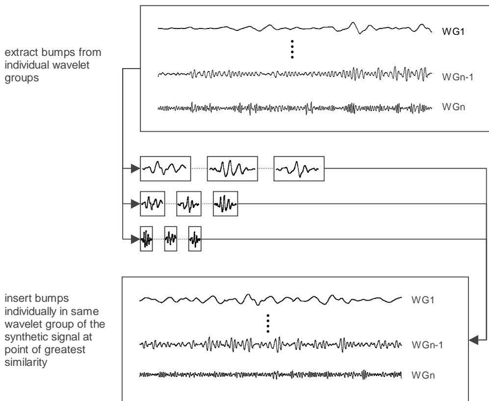
Figure 6) Nonsynchronised bump reinsertion procedure.
