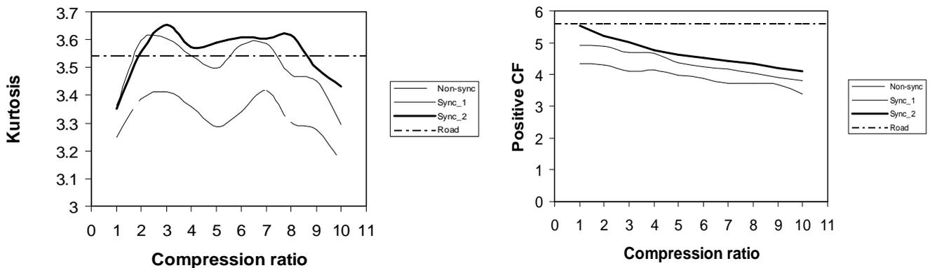
Figure 11) Kurtosis and Crest Factor variation (average of five runs) as a function of the signal compression ratio for a data set from a Renault automobile.
