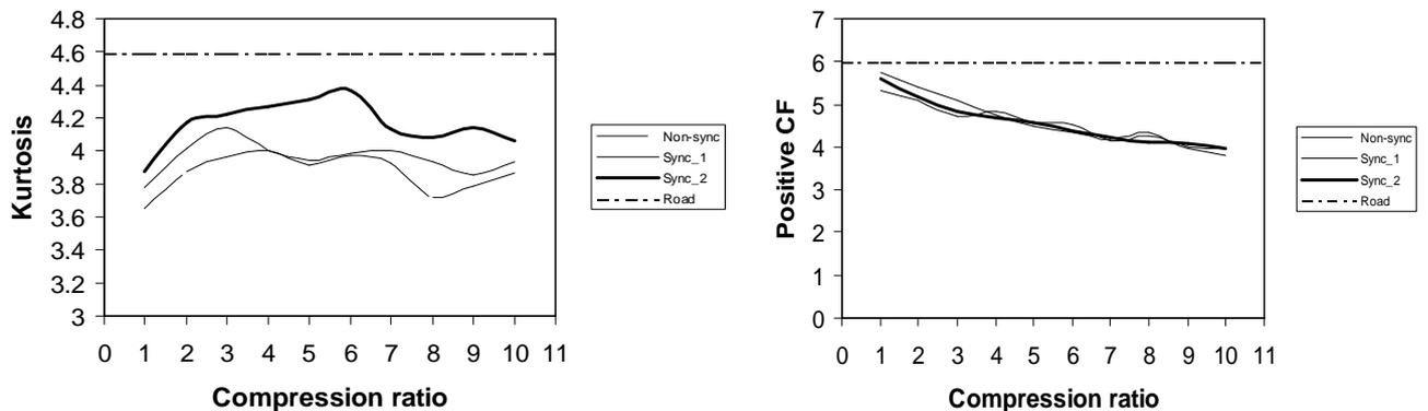
Figure 12) Kurtosis and Crest Factor variation (average of five runs) as a function of the signal compression ratio for a data set from a BMW automobile.
