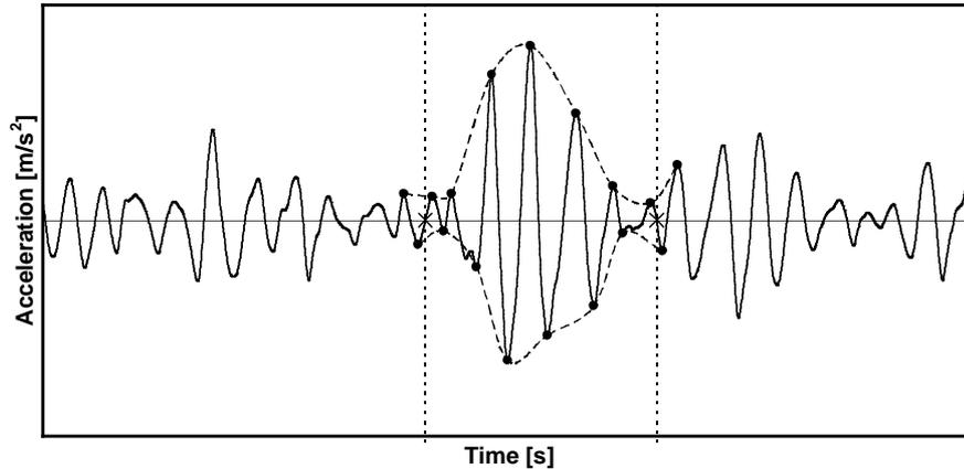
Figure 5) Bump selection by means of trigger level and end inversion check.
