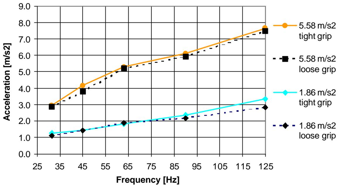
Figure 5) Average equal sensation curves from the tests using the 63 Hz reference signal.
