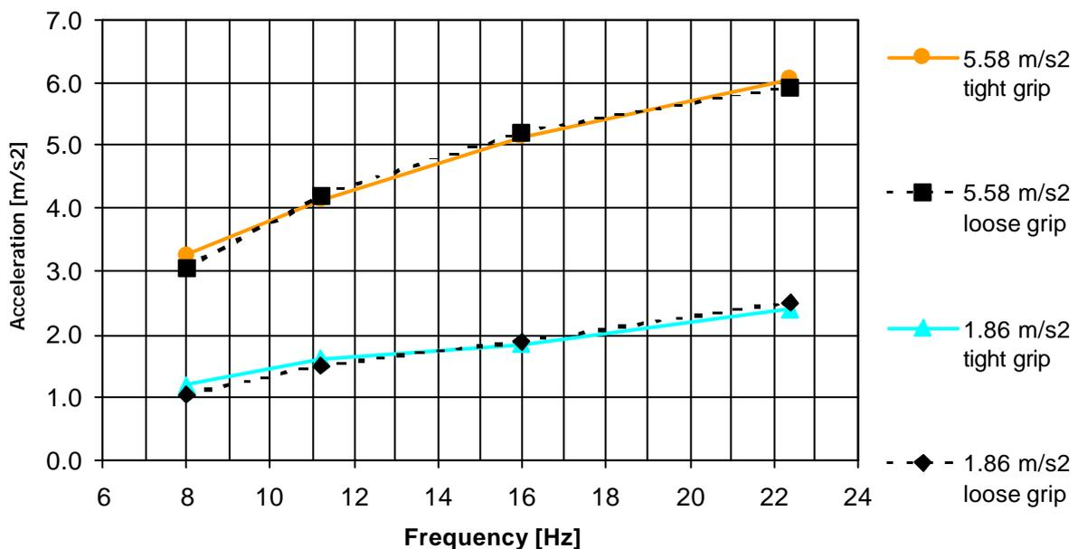
Figure 4) Average equal sensation curves from the tests using the 16 Hz reference signal.
