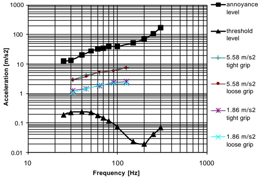
Figure 6) Comparison between the equal sensation curves determined using the 63 Hz reference sinusoid and threshold and annoyance curves [20] for the vertical direction of a vibrating handle.
