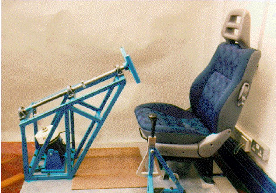
Figure 1) Steering wheel rotational vibration test rig.
