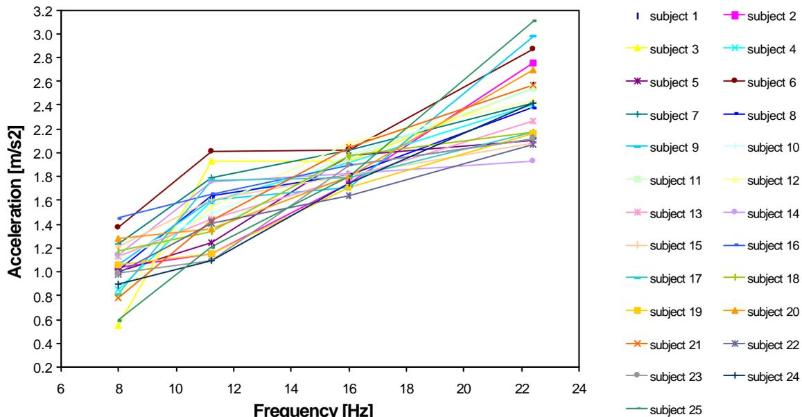
Figure 3) Results from all subjects obtained using the 16 Hz reference signal at 1.86 m/s<sup>2</sup> with loose grip.
