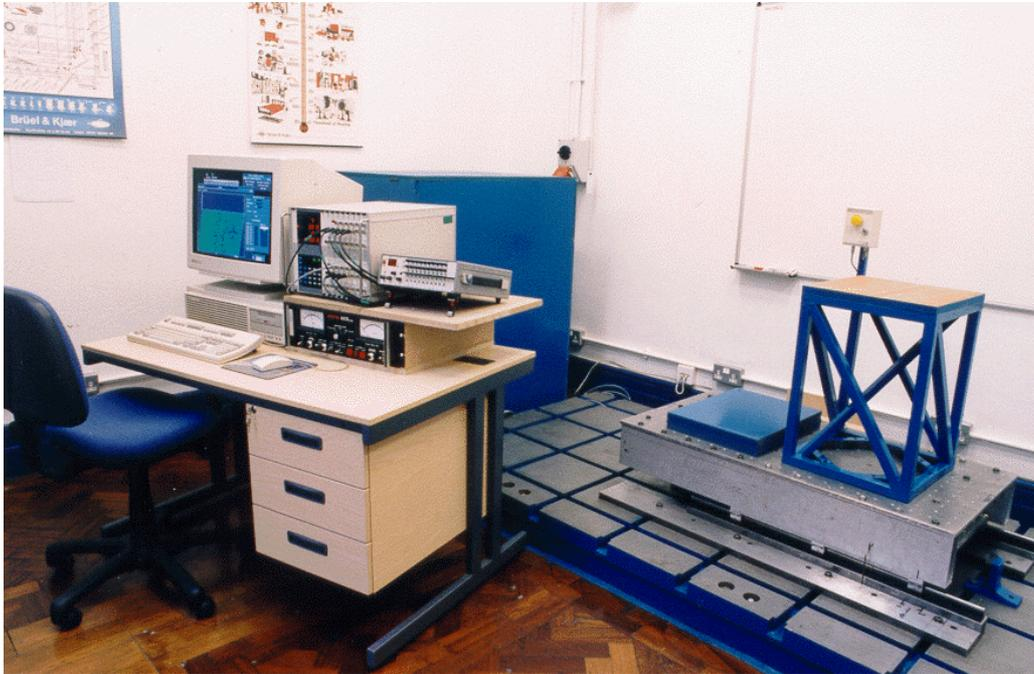
Figure 1) For-aft direction whole-body-vibration test rig.
