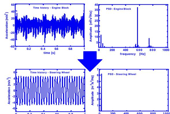
Fig. 4 – Transmission of vibration to wheel.
