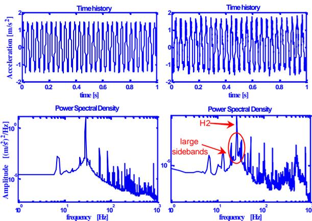
Fig. 5 – Regular and irregular idle vibrations.
