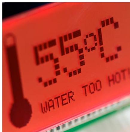
Figure 4) Example of a cognitively intuitive design: “*Bathe Safe*” by Oliver Wooderson utilises a large colour screen to monitor bath temperature to avoid the dangers of scalding. Colours, typography and visuals combine to render the situation cognitively obvious.
