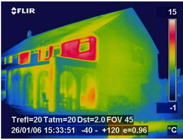
Thermal image of a house – use of new technology to understand heat losses (Joseph Hodgkinson, MadeinBrunel Innovation Show, 2006).
