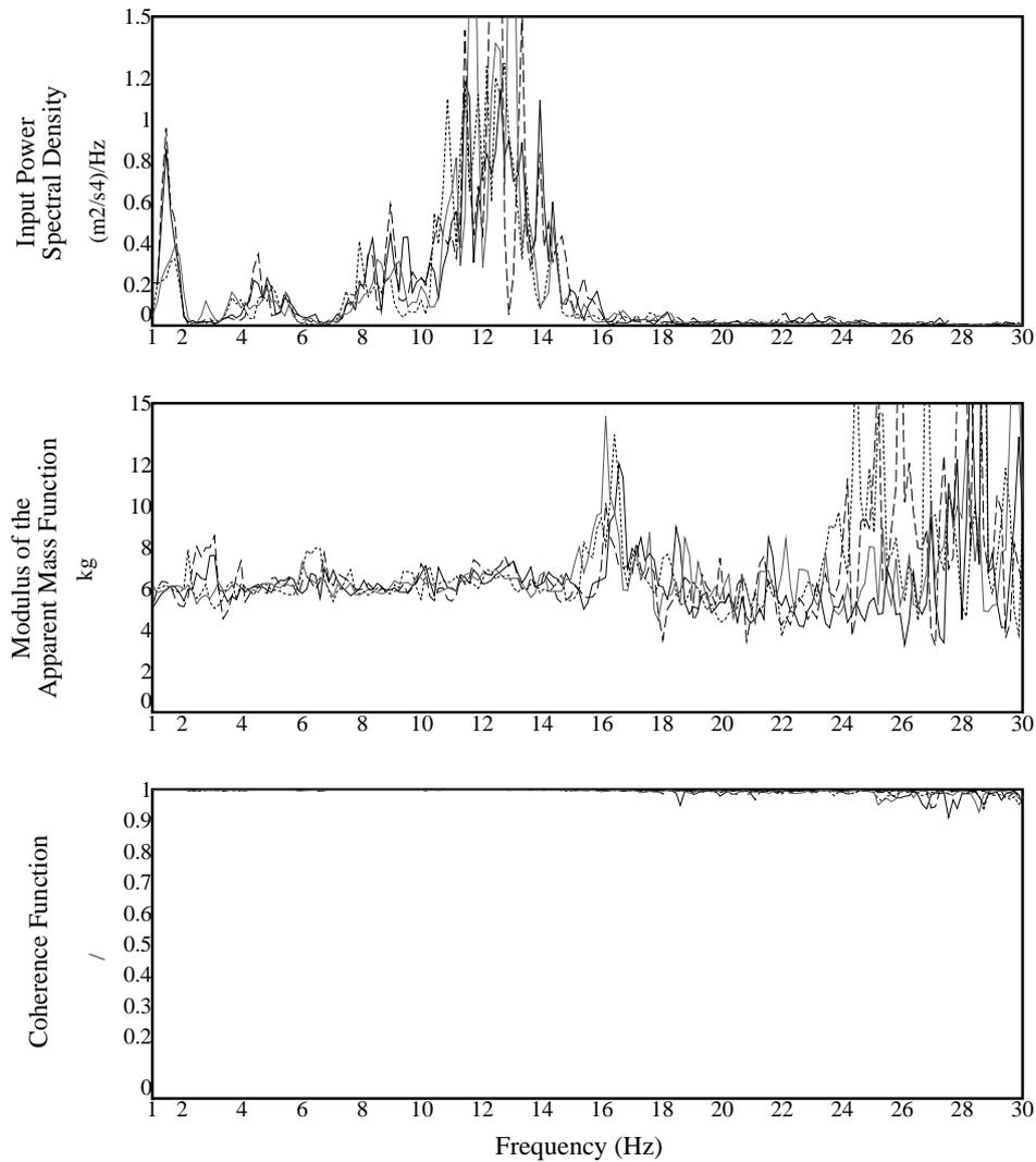
Figure 8) Apparent mass results from the 4 runs over the pave' surface with the 5.67 kg mass.
