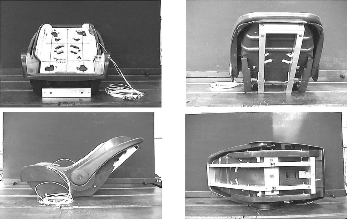
Figure 7) Four views of the child seat and apparent mass sensor.
