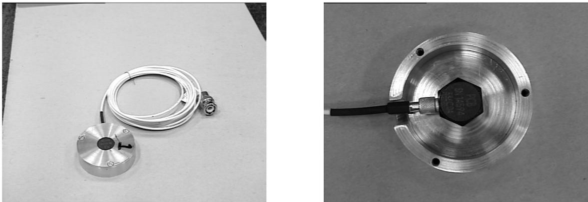
Figure 5) Two views of the child-bar used for testing child seats.
