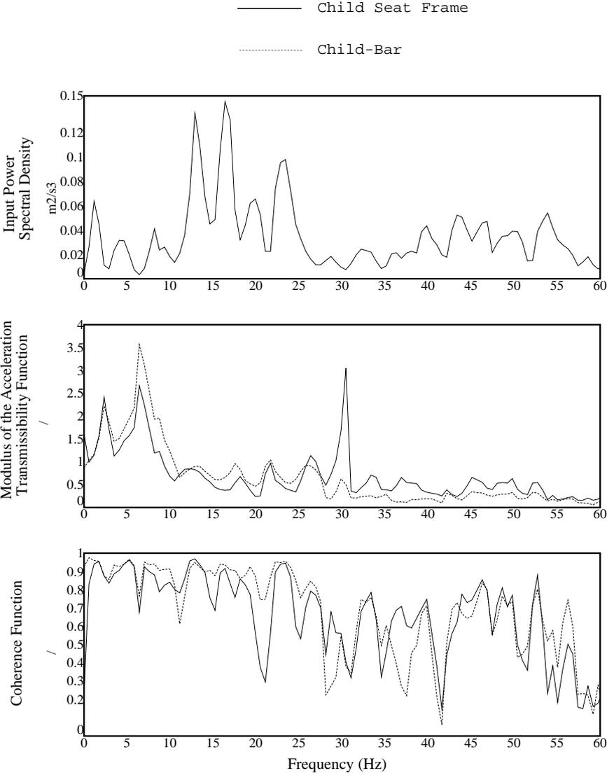
Figure 5) Input acceleration power spectral density, acceleration transmissibility function and coherence function for one run over the pave' surface with the seat of Figure 1.
