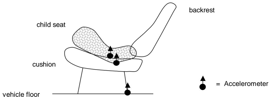
Figure 4) Accelerometer layout used for road testing.
