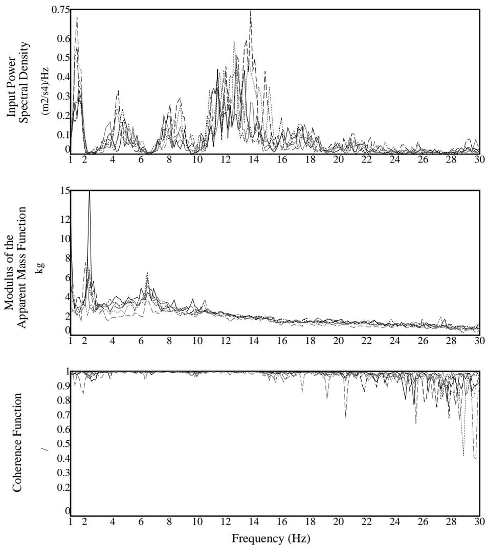
Figure 9) Apparent mass results from the 6 runs over the pave' surface with the child.
