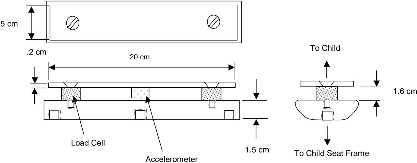
Figure 6) Apparent mass sensor for use in child seats.
