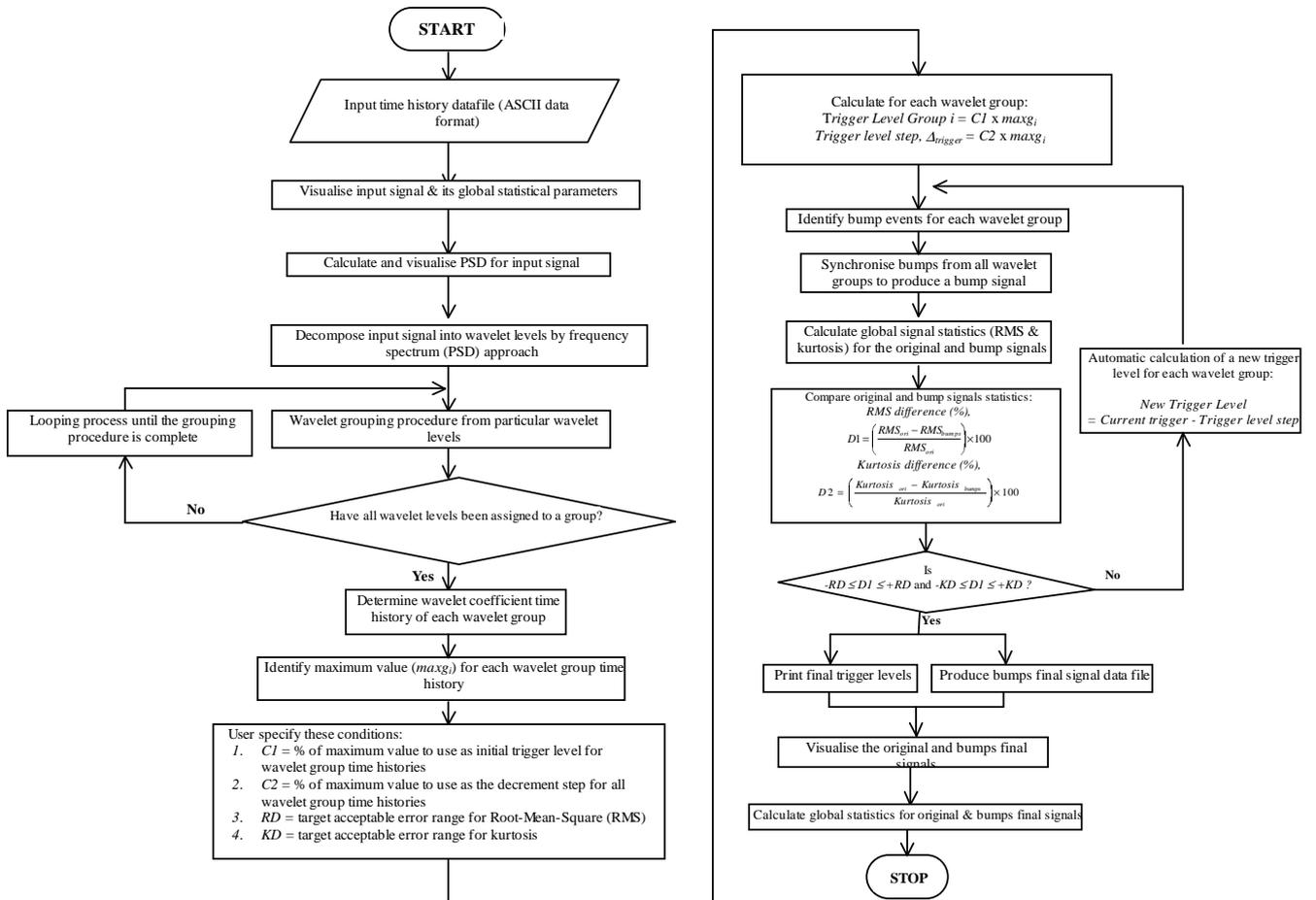
Figure 1: A flowchart of the WBE algorithm
