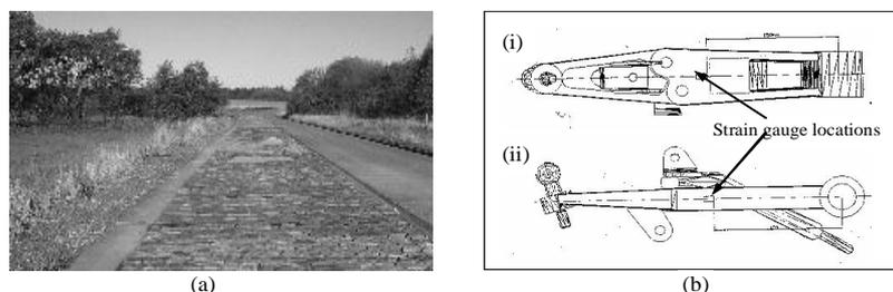
Figure 4: (a) Pavé test track used for the road tests, (b) Schematic view of strain gauge locations on the component for: i) tensile mean loading, ii) compressive mean loading [8]
