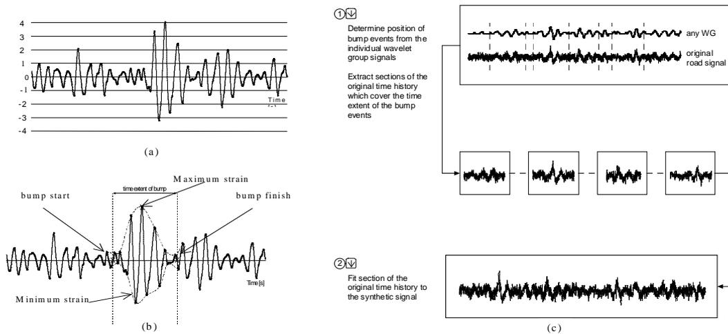
Figure 2: (a) Bump identification using trigger levels, (b) Decay enveloping of a bump event, (c) Schematic diagram of bump synchronisation
