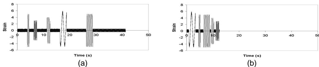
Figure 3: Plots of the test signal: (a) original signal (*no. of data points,  $n = 16000$ ,  $RMS = 1.51$ , kurtosis,  $K = 7.37$* ); (b) bump signal ( *$n = 4997$ ,  $RMS = 2.62$ ,  $K = 2.53$* )
