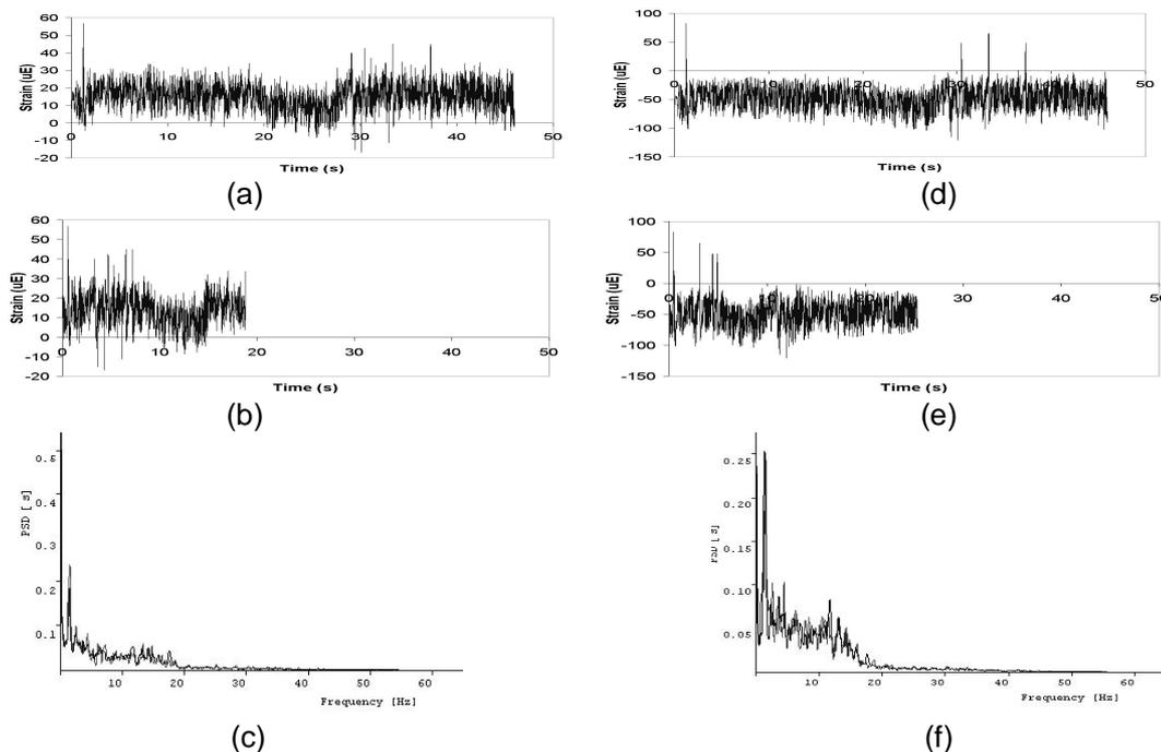
Figure 5: Plots for S1: (a) original signal ( $n = 23000$ ,  $RMS = 7.0$ ,  $K = 3.4$ ); (b) bump signal ( $n = 9413$ ,  $RMS = 7.8$ ,  $K = 3.6$ ); (c) PSD of the original signal (black colour) and bump signals. Plots for S2: (d) original signal ( $n = 23000$ ,  $RMS = 19.0$ ,  $K = 3.8$ ); (e) bump signal ( $n = 12674$ ,  $RMS = 21.0$ ,  $K = 4.0$ ); (f) PSD of the original signal (black colour) and bump signals
