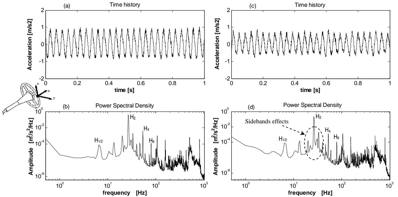
**Fig. 3** Steering wheel idle vibration signature along the vertical (z) axis. Weakly modulated condition: (a) time history and (b) its relative PSD. Strongly modulated condition: (c) time history and (d) its relative PSD.
