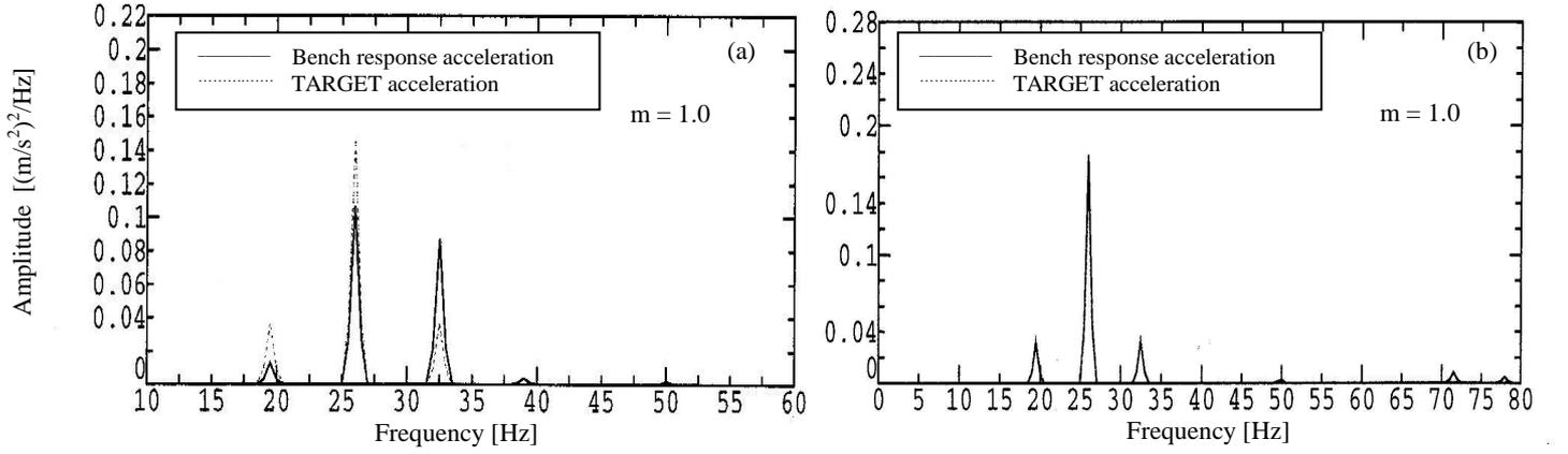
**Fig. 2** – Test signals: (a) comparison between target and bench response acceleration before compensation; (b) comparison between target and bench response acceleration after compensation.
