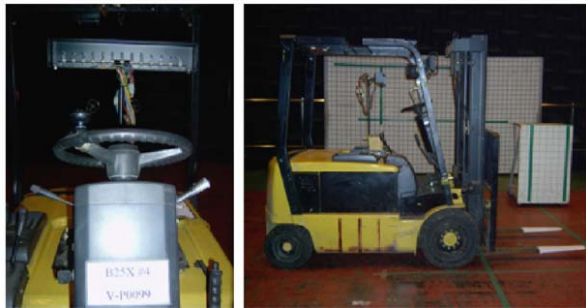
Fig. 6 Set up of the light bulb shadow test (Chin-Bong et al., 2008)
