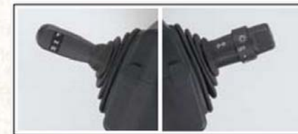
Fig. 28 Electric shift lever & Automotive style light switch (Toyota Lift of Minnesota, 2010)
