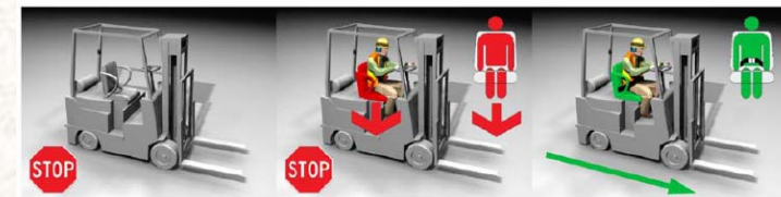
Fig. 21 Schematic view of the seatbelt system operation (Horberry et al., 2004)
