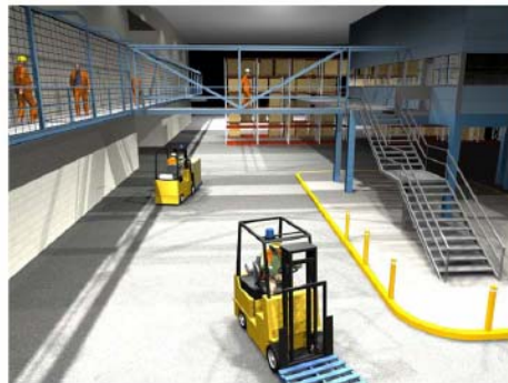
Fig. 15 Computer generated image of a possible environment for forklift pedestrian separation (Horberry et al., 2004)
